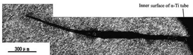
Fig. 6 Montage of optical micrographs of the crack along a shear band
